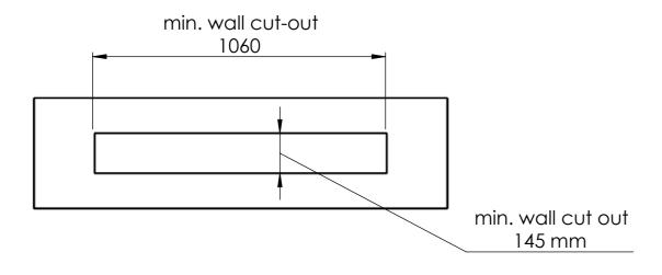
Mounting if top plate is to rest on top of surrounding surface Note: base plate can get hot! Ensure that the surrounding surface can withstand a temperature of around 50 degrees C.
